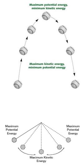
The change of potential energy into kinetic energy, and kinetic energy into potential energy, in a pendulum.
